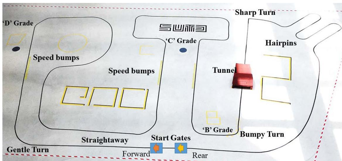
**Figure 1.** Layout of the line-following track with obstacles. It is designed with increasing difficulty as the track progresses clockwise.
