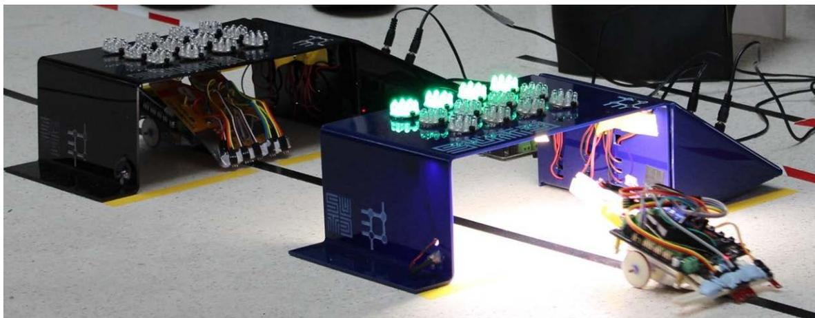
**Figure 2.** The intelligent start boxes (left: rear, right: forward) with exterior status and interior start LEDs.
