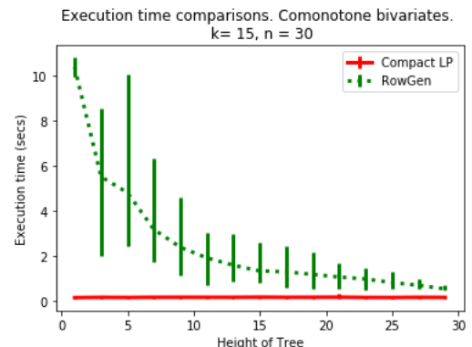
Figure 9 Execution times (in secs) of compact LP and row generation for various tree heights, n=30 , k=15
