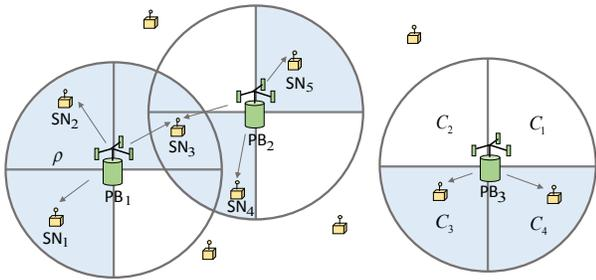
Fig. 1. System model of AD-WPT (illustrative example of  $N = 4$ ). The circular areas with radius  $\rho$  are the charging regions of the PBs. The shaded sectors in the charging regions are the active sectors of the PBs.
