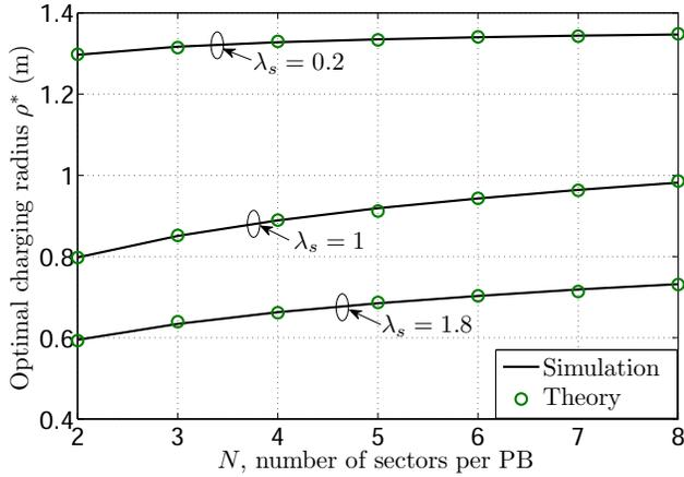
Fig. 3. Optimal charging radius  $\rho^*$  for average power maximization versus  $N$  ( $\lambda_p = 0.1$ ,  $P_p = 10$  W and  $\alpha = 3$ ).
