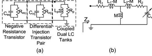
Fig. 2. Equivalent circuit (a) ILFD AC half circuit and, (b) series equivalent of coupled dual LC tank.
