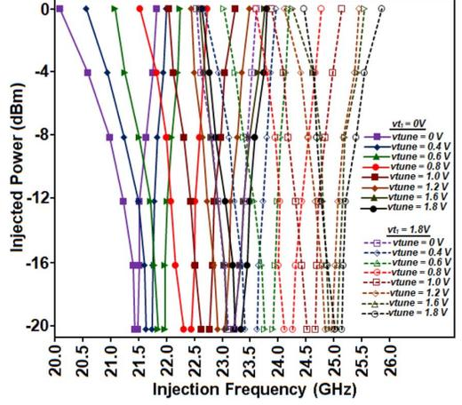
Fig. 4. Measured input sensitivity of ILFD.
