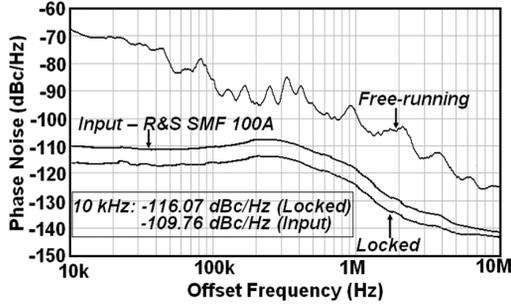
Fig. 6. Measured ILFD phase noise.
