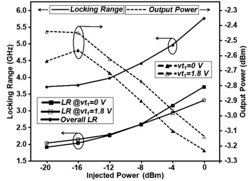
Fig. 5. Measured locking range and output power.
