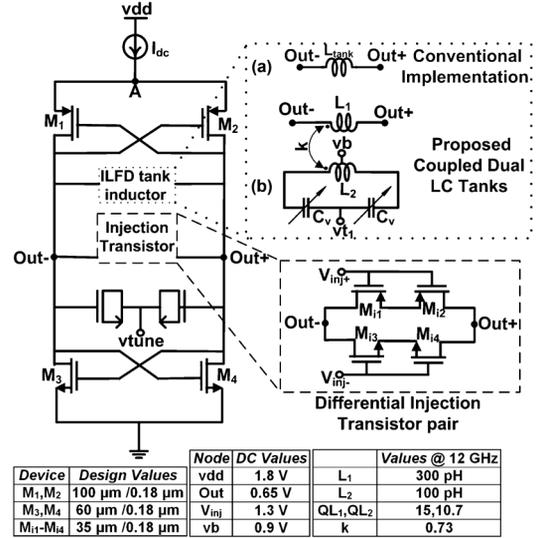
Fig. 1. Schematic of injection locked divide-by-2 divider.
