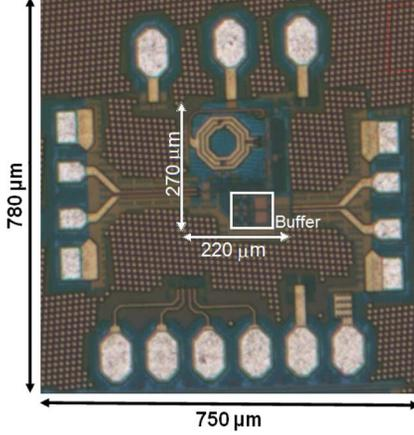
Fig. 3. Die microphotograph of ILFD.
