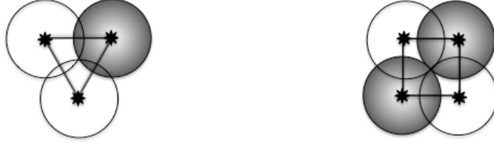
Fig. 1. Examples of “tight” plane tiling with low sensor overlap (i.e. low F_{\max} )
