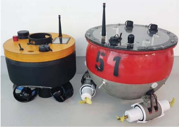
Fig. 3. The two robotic platforms: the new buoy design v2 (left) side by side with one of the previous buoy model v2 (right).
