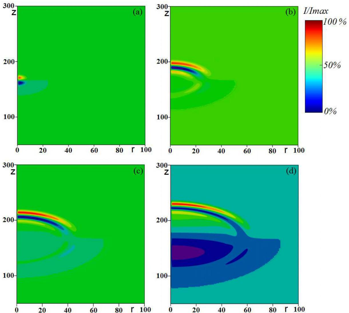
FIG. 1. Three-dimensional electromagnetic pulse intensity  $I(r, z, t) = E^2(r, z, t)$  at different instants of time ( $\alpha = 0.005$ ,  $\beta = -1$ ,  $\chi = 0.1$ ,  $\Gamma = 0.1$ ): (a) initial pulse; (b)  $t = 2 \times 10^{-13}$  s; (c)  $t = 5 \times 10^{-13}$  s; and (d)  $t = 7 \times 10^{-13}$  s.
