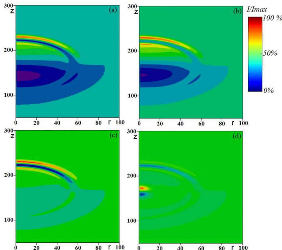
FIG. 3. Three-dimensional electromagnetic pulse intensity  $I(r, z, t) = E^2(r, z, t)$  for different values of the parameter  $\alpha$  ( $t = 7 \times 10^{-13}$  s,  $\Gamma = 0.1$ ): (a)  $\alpha = 0.0$ ; (b)  $\alpha = 0.1$ ; (c)  $\alpha = 0.5$ ; and (d)  $\alpha = 1.0$ .
