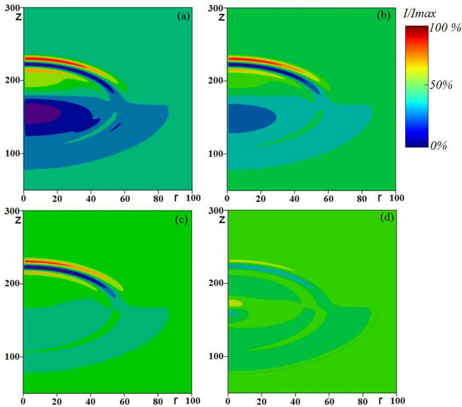
FIG. 2. Three-dimensional electromagnetic pulse intensity  $I(r, z, t) = E^2(r, z, t)$  for different values of the relaxation rate  $\Gamma$  ( $t = 7 \times 10^{-13}$  s,  $\alpha = 1$ ,  $\beta = -1$ ): (a)  $\Gamma = 0.01$ ; (b)  $\Gamma = 0.02$ ; (c)  $\Gamma = 0.05$ ; and (d)  $\Gamma = 0.1$ .
