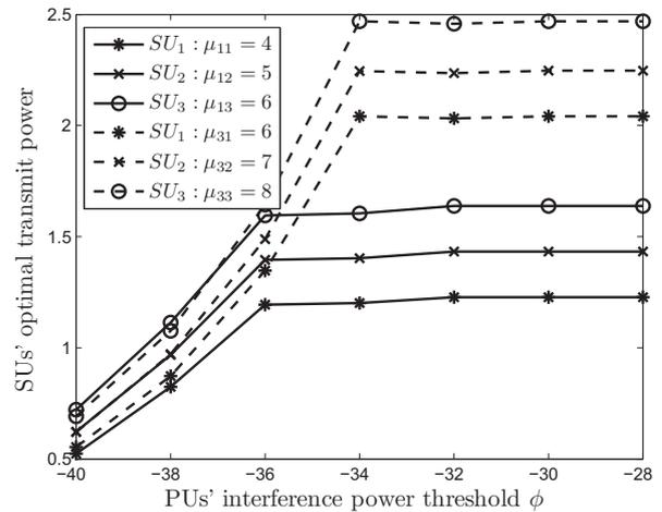
Fig. 4: SUs' transmit power updates according to  $\phi$ .
