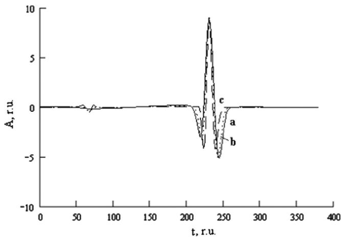
**Fig. 3.** Dependence of the pulse on time for different values of the pulse velocity at the inlet of the specimen. All the quantities are scaled in relative units (r.u.). Curve (a) corresponds to  $v=0.9$ , (b) to  $v=0.95$ , and (c) to  $v=0.99$ .
