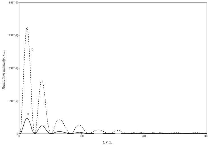
Fig. 3. Dependence of the dipolar radiation intensity on time ( $\Delta = 0.05$ ): (a)  $r = 4$  and (b)  $r = 4.4$ .
