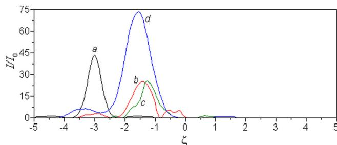
FIG. 4. Intensity distribution  $I(\nu_0, \zeta, \tau)/I_0$  of the pulse field in an array of CNTs in a cross-section parallel to the plane  $\xi O \xi$  ( $\xi = x\omega_0/c$ ,  $\zeta = z\omega_0/c$ ) and passing through the point with coordinates  $\nu = \nu_0$ , when the laser pulse is reflected from a region of elevated electron density at different instants of the dimensionless time  $\tau$ : (a)  $\tau = 0$ , (b)  $\tau = 4$ , (c)  $\tau = 8$ , (d)  $\tau = 12$ .
