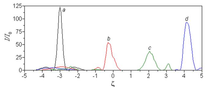
FIG. 2. Intensity distribution  $I(\nu_0, \zeta, \tau) / I_0$  of the pulse field in an array of CNTs in an area parallel to the plane  $\zeta O\zeta$  ( $\xi = x\omega_0/c$ ,  $\zeta = z\omega_0/c$ ) and passing through the point with coordinates  $\nu = \nu_0 = 0$ , at different instants of the dimensionless time  $\tau$ : (a)  $\tau = 0$ , (b)  $\tau = 4$ , (c)  $\tau = 8$ , (d)  $\tau = 12$ .
