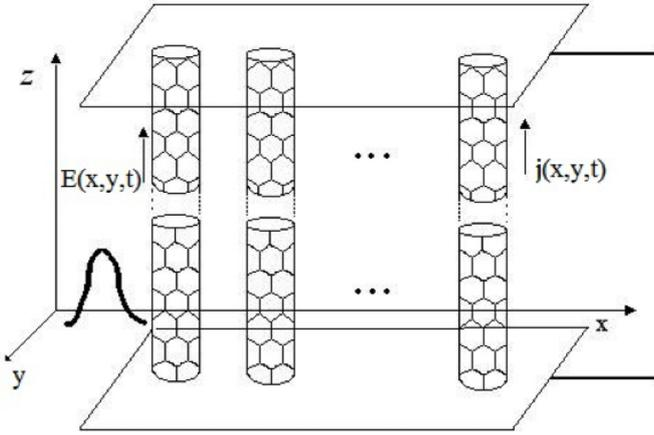
**Fig. 1.** Geometry of the problem with carbon nanotubes aligned along the  $z$ -direction and contributing to generating a Bragg grating along the  $x$ -direction.
