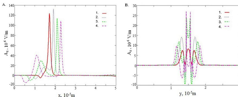
**Fig. 3.** (A) Spatial variations of the (vector potential) electric field at four consecutive instants in time. In the presence of the Bragg grating, results are given for (1A)  $t = T_0$ , (2A)  $t = 2T_0$ , (3A)  $t = 3T_0$ , (4A)  $t = 4T_0$ . The dependence of the electric field on the transverse coordinate,  $y$ , is presented on (B).
